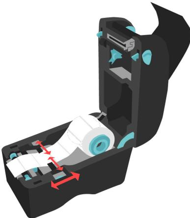
3. Using the Media Guide Adjuster Knob, adjust the Media Guide until it is flush but not tight against the media.
