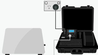
*Note: Because the power test is not specified in the AS/NZS 3760:2022 standard, there is no pass/fail value built in to the tester. It is up to the user to determine if the item is a pass or a fail based on the compliance/name plate.*
