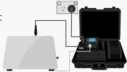
If the result was a **PASS** - Tag with PASS tag showing "next test due" date and return the device to service.
