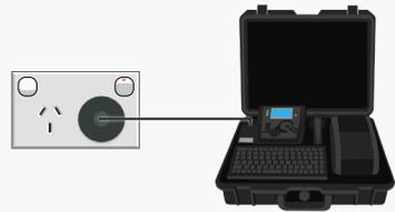
*Testing Portable RCDs with no physical switch*
