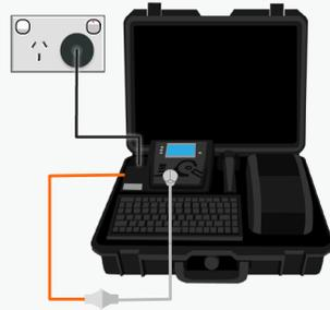
If the result was a **PASS** - Tag with PASS tag showing "next test due" date and return the device to service.
