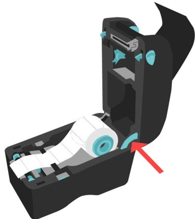
4. To shut the printer, push the support hinge in, then gently shut the printer, ensuring it latches shut. Press the Feed button on the printer before printing, to ensure the tag is printed correctly.
