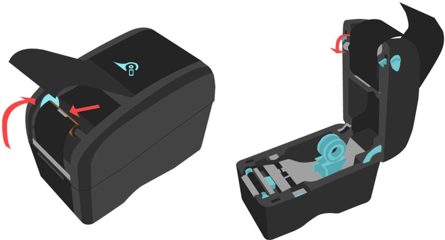
6. Attach the ribbon to the empty roll using a piece of tape - try to attach the ribbon as straight as possible.
