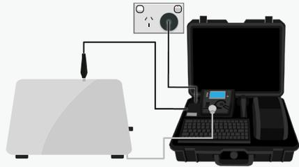
If the result was a **PASS** - Tag with PASS tag showing "next test due" date and return the device to service.
