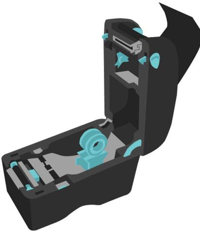
3. Open the printer and get the thermal transfer ribbon ready. Ensure the ribbon unwinds from underneath as shown in Step 5
